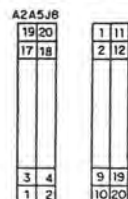
HF-8054A Receiver (622-3475-210), Cabling, Connector Layout and Pin Numbering Figure 4A
